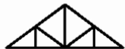
Waddell "A" Truss
