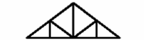
Waddell "A" Truss
